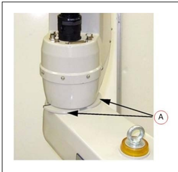
Figure 5-15. Joint 2 Adjustable Hardstop Plates installed in Position 2 (A)
