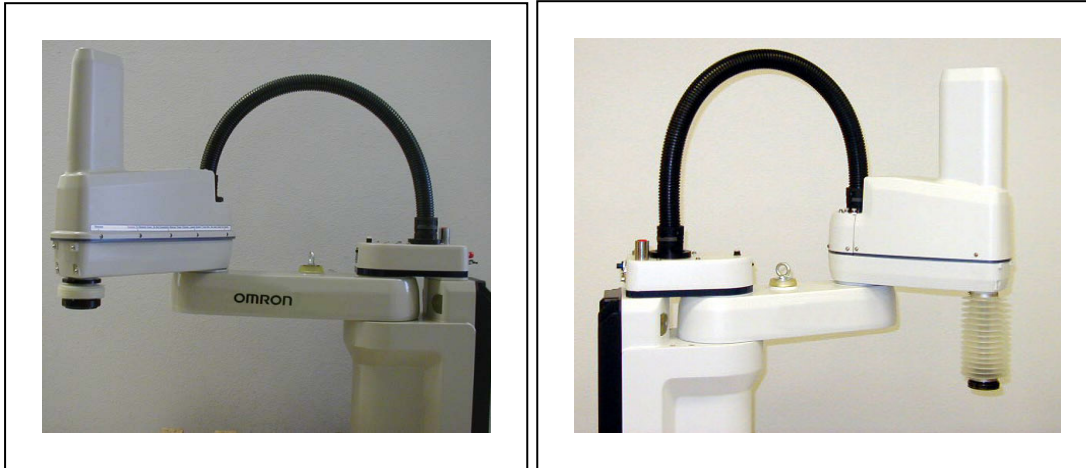
Figure 1-5. IP65 Version (left), Cleanroom Version (right)
