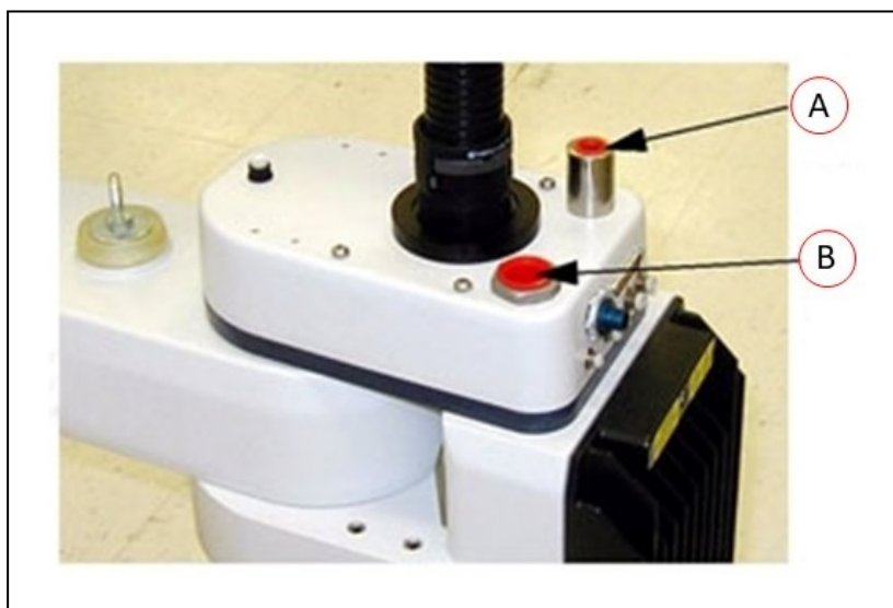
Figure 10-2. Compressed Air Inlet Port - ⅜ inch NPT Female fitting (A), High Flow, Low Vacuum Port - ¼ inch NPT Female Fitting (B)
