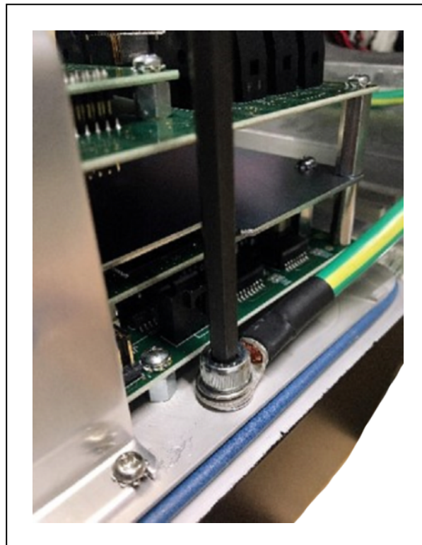
Figure 7-12. Removing Ground Screw Wire on iCS-ECAT Chassis with 5 mm Hex Wrench
