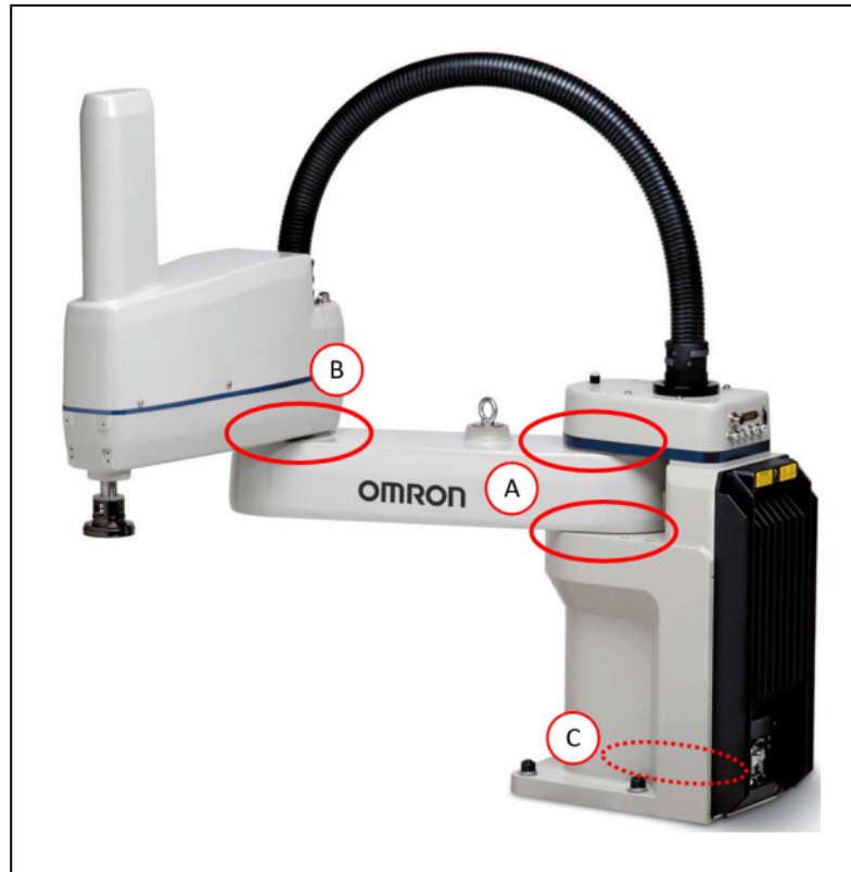
Figure 7-5. eCobra Oil Leak Inspection Areas
