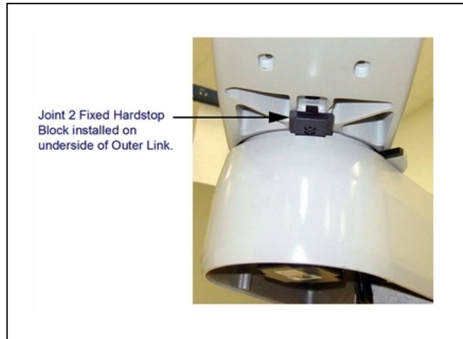
Figure 5-17. Fixed Hardstop Block for Joint 2 installed on underside of Outer Link
