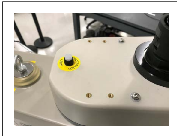
Figure 5-2. External Equipment Mounting Location, J1
