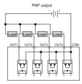
This unit is equipped with 4 pulse output terminals. The common terminal is used commonly The terminal is the push-in type. Also read "Cautions when connecting the Push-In Plus terminal
