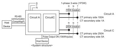
To measure, you first need to make settings in the settings mode for the circuits and communications.
