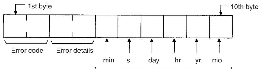
The time stamp is provided in the CVM1-DRM1-V1 Master Unit only. These bytes will be all zeros for the C200HW-DRM1-V1 Master Unit. (The program can be used to manually attach a time stamp to the error log records by using the clock in the CPU Unit for C200HX/HG/HE and C200HS PLCs.)
