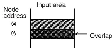
To eliminate the I/O area overlap and clear this error, change the node address setting on one of the Slaves as shown below and restart the Master by turning the power OFF and ON again or restarting.
