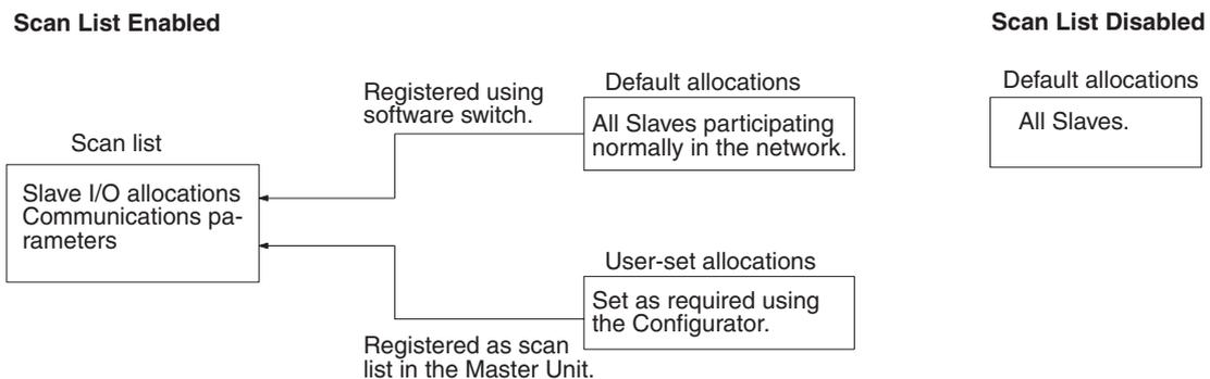
**Note** The scan lists created with the Configurator will be needed again for registration in the Master Unit if the Master Unit is ever set to disable the scan list or if the Master Unit is replaced. Be sure to save any scan lists you create with the Configurator as network files or master parameter files.
