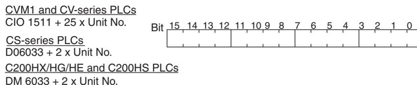
The current communications cycle time is stored in the above word as 4-digit BCD in ms. The value is truncated at the decimal point. The value is refreshed each PLC execution cycle for CS-series, C200HX/HG/HE, and C200HS PLCs; it is refreshed each peripheral servicing time for CVM1 and CV-series PLCs.
