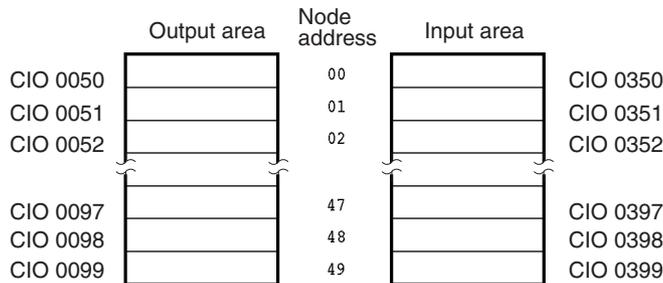
With the CS Series, the default DeviceNet Output Area (CIO 0050 to CIO 0099) is within the I/O Area (CIO 0000 to CIO 0319). For this reason, in systems with a large number of I/O points, where CIO 0050 to CIO 0099 would be allocated to I/O Units, ensure that there is no overlap of area allocation using one of the following methods.
