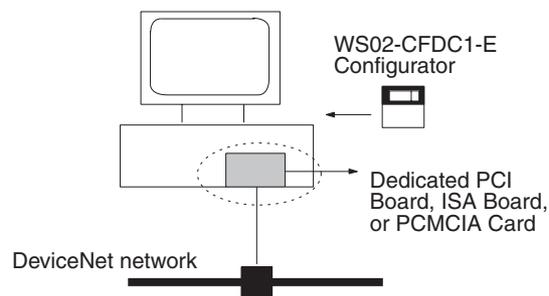
The Configurator is treated as one DeviceNet node.
