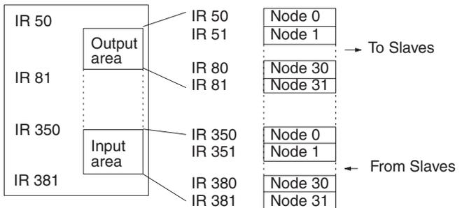
**Note** With the CS1 Series, the DeviceNet Output Area (CIO 0050 to CIO 0099) is contained inside the I/O Area (CIO 0000 to CIO 0319). For this reason, in systems with a large number of I/O points, edit the I/O table with the CX-programmer so that no actual I/O points (in Basic I/O Units) are allocated to the words between CIO 0050 and CIO 0099.
