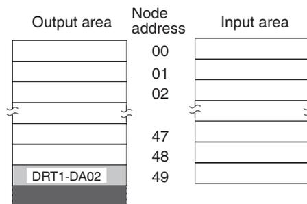
To eliminate the above problems and clear this error, change the node address setting on the Slave and restart the Master by turning the power OFF and ON again or restarting.
