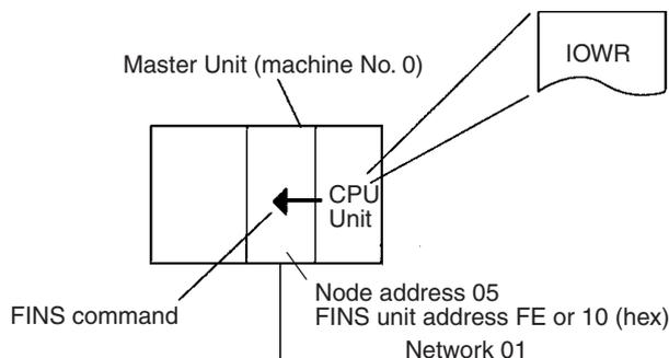
The program reads 20 records of error log data from the Master Unit, stores the data, and then clears the error log. This process is repeatedly executed. The ERROR LOG READ (21 02) and ERROR LOG CLEAR (21 03) commands are used.
