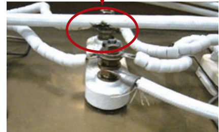
The area within the red circle is the location of the short-circuit.
