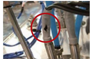
The area within the red circle is the location of the short-circuit.
