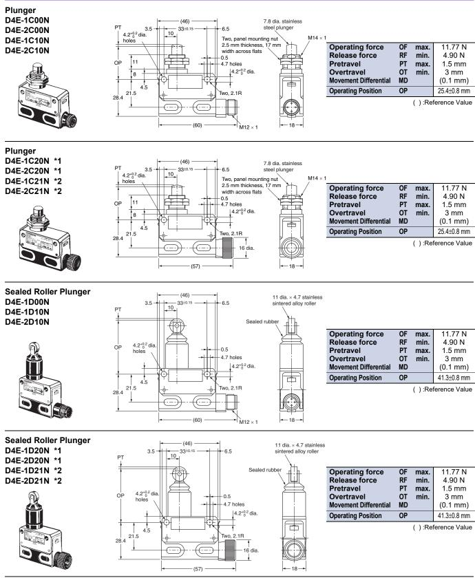
Note: Unless otherwise specified, a tolerance of  $\pm 0.4$  mm applies to all dimensions.
