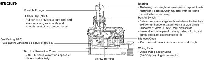
Screw terminal incorporates a M3 screw with a toothed washer.
