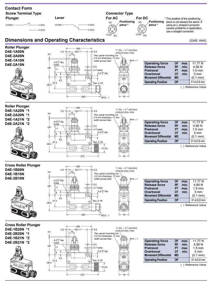
Note: Unless otherwise specified, a tolerance of  $\pm 0.4$  mm applies to all dimensions.
