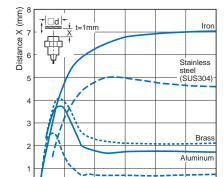
20 30 40 50 60 Side length of sensing object: d (mm)
