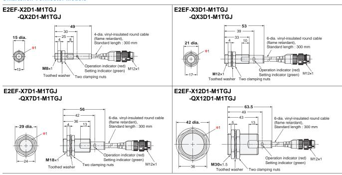
\*1. The E2EF-QX□D type Clamping nut (optional accessory) is grooved to identify the material (SUS303, with fluororesin coating).
