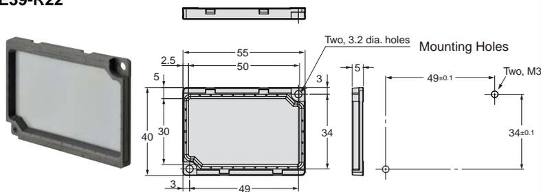
Materials Reflective surface: Methacrylic resin (PMMA)
