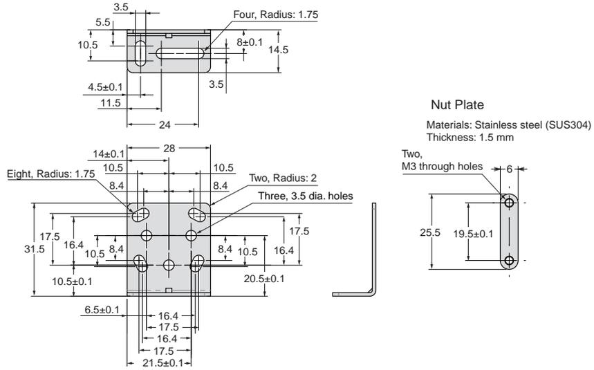
**With E39-L190 Mounting Bracket Attached for Bottom Mounting**
