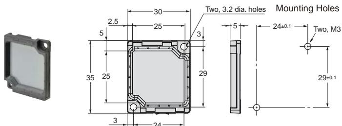
Materials Reflective surface: Methacrylic resin (PMMA)
