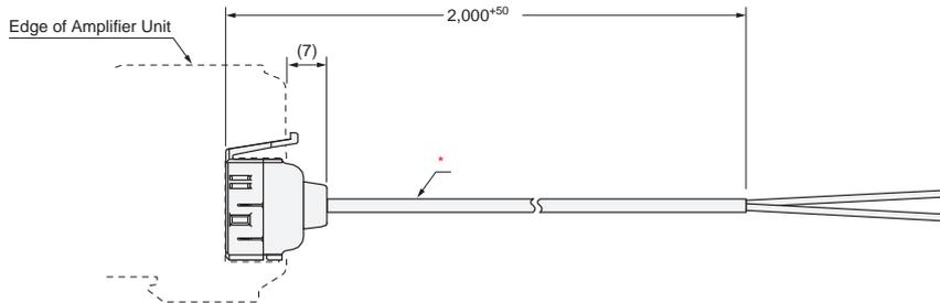
\*4-dia. cable with 2 conductors, Standard cable length: 2 m (Conductor cross-section: 0.2 mm<sup>2</sup> (AWG24), Insulation diameter: 1.1 mm)
