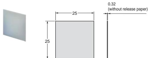
Materials Methacrylic resin (PMMA)
