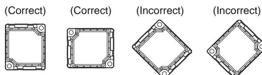
Sheet products (E39-RS10/E39-RS11) are peel-off stickers. Peel off the release paper and apply the sheet to a flat surface for installation. If there are any dirt and dust on the installation surface, a reduction in adhesion and deflection of a sheet may occur, resulting in malfunction.
