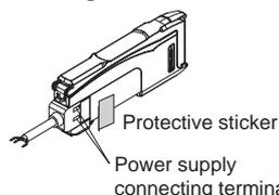
Amplifier Unit with Connector for Sensor Communications Unit
