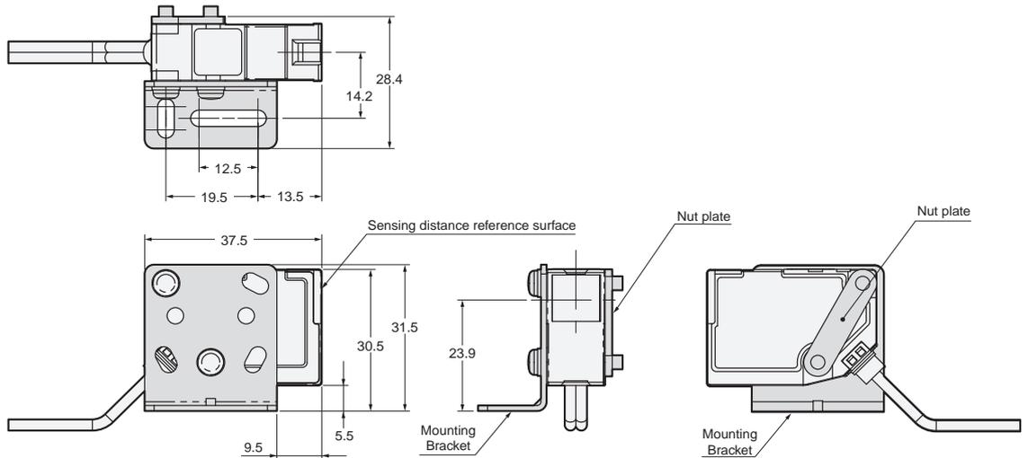
**With E39-L190 Mounting Bracket Attached for Back Mounting**
