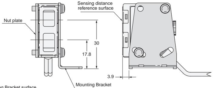
\* When adjusted, the adjuster extends 0.8 mm from the Mounting Bracket surface.
