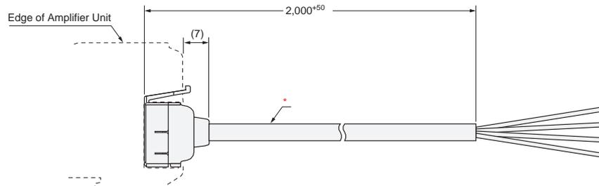
\*4-dia. cable with 4 conductors, Standard cable length: 2 m (Conductor cross-section: 0.2 mm<sup>2</sup> (AWG24), Insulation diameter: 1.1 mm)
