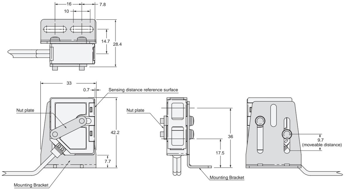
**With E39-L186 Mounting Bracket Attached for Back Mounting**
