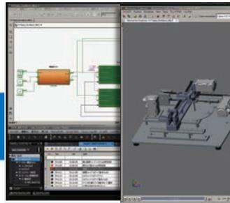
Complex feedback control that is designed with MATLAB®/Simulink® can be imported into programs.
