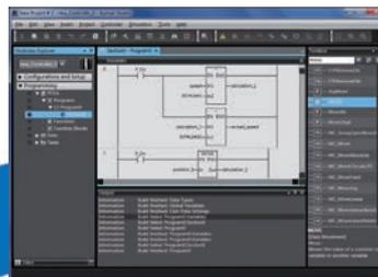
One Integrated Development Environment software Sysmac Studio is fully compliant with the open standard IEC 61131-3. Programming with variables eliminates the need to learn the internal memory map of the PLC and allows the programs to be reused.
