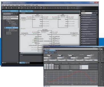
Advanced motion control applications can be created quickly just by combining PLCopen® Function Blocks for Motion Control.
