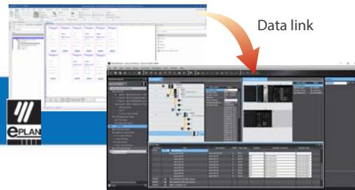
Circuit diagrams designed using electrical CAD data (e.g., unit configurations and signal lines) can be imported to the Sysmac Studio and automatically reflected in unit configurations and settings and allocated variables.
