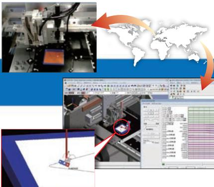
Movement of the machine connected online can be displayed on the CAD in real time, and movement can also be reproduced from the trace data. Maintenance and troubleshooting can be performed in remote locations.
