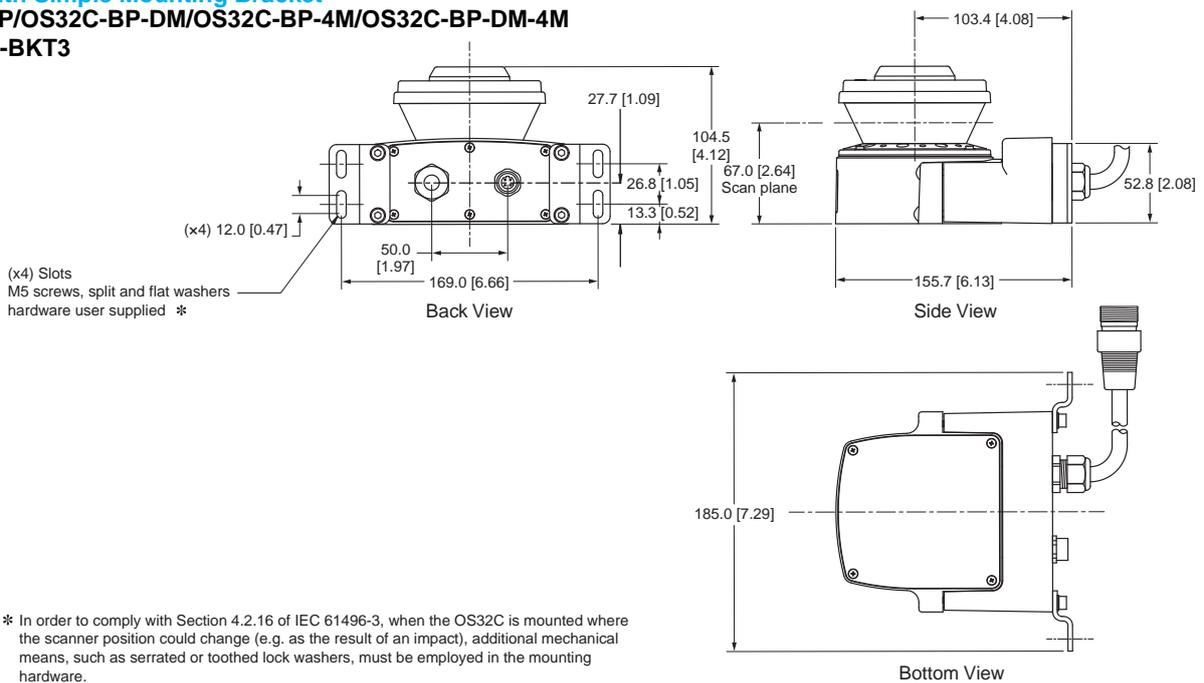
\* In order to comply with Section 4.2.16 of IEC 61496-3, when the OS32C is mounted where the scanner position could change (e.g. as the result of an impact), additional mechanical means, such as serrated or toothed lock washers, must be employed in the mounting hardware.
