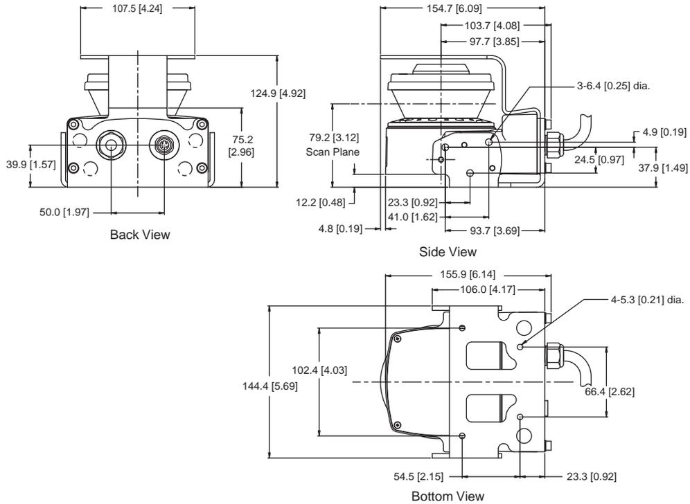
OS32C with Bottom/Side Mounting Brackets and XY Axis Rotation Mounting Kit
