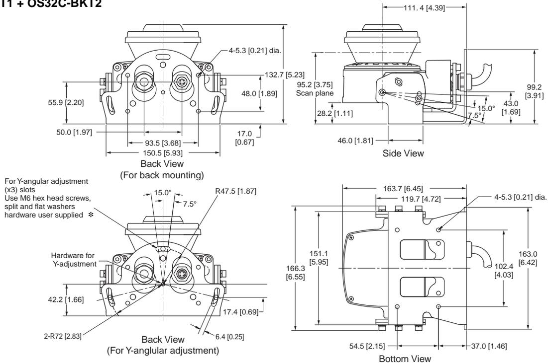
\* In order to comply with Section 4.2.16 of IEC 61496-3, when the OS32C is mounted where the scanner position could change (e.g. as the result of an impact), additional mechanical means, such as serrated or toothed lock washers, must be employed in the mounting hardware.
