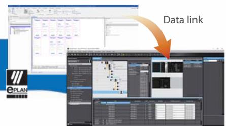
Circuit diagrams designed using electrical CAD data (e.g., unit configurations and signal lines) can be imported to the Sysmac Studio and automatically reflected in unit configurations and settings and allocated variables. Seamless and accurate setup using electrical CAD design data speeds up the engineering process and improves design efficiency.
