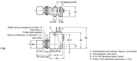
Note: The Operation Unit can be inserted and removed.
