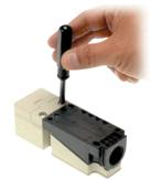
When positioning the sensing surface to the side, rotate it to the required position, then fit it into the case. The possible positions are 0, 90, 180, and 270°. Do not forcefully rotate the sensing surface.
