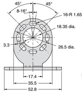
Material: Stainless steel (Top/bottom mounting brackets, hexagon socket head cap screws)
