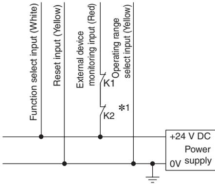
K1, K2: Relay or other device that controls hazardous parts of the machine
