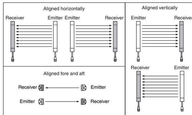
If 2 sets are installed near each other, reflection from the surfaces may cause mutual interference.
