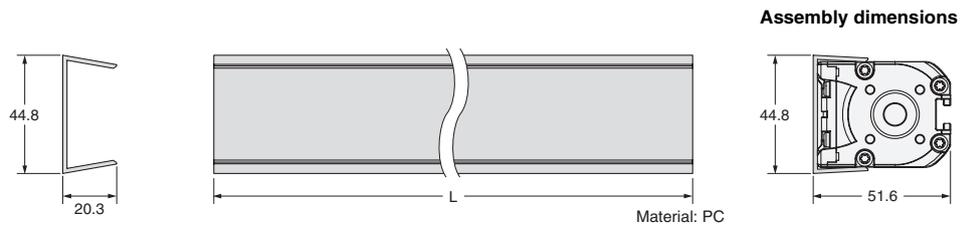
When protective height is 0190 to 1790 mm: L = □□□□ - 20 mm
