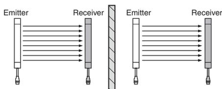
2. Alternate the direction of emission between 2 sets (alternation)
