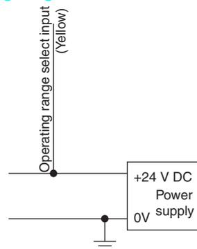
**Make sure to connect the operating range select input line to 24 V or 0 V according to the distance used. Leaving the wiring open without connection will result in wiring error and the F3SR-B will enter lockout. If the wiring at startup is open or wiring is switched during operation, the F3SR-B enters lockout.**
