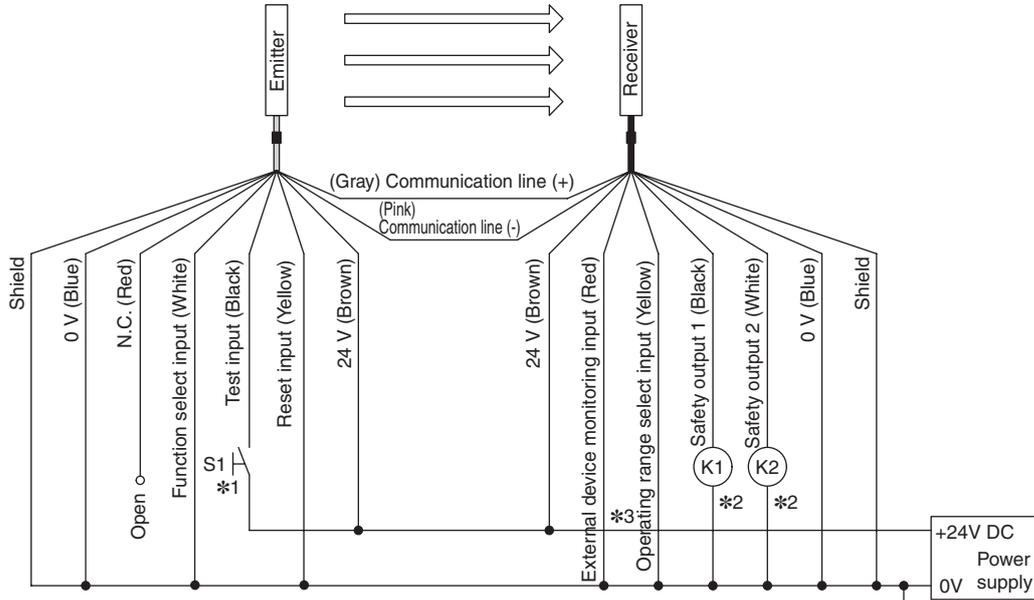
S1 : External test /lockout reset switch (connect to 0V if a switch is not required)
