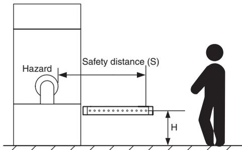
Use  $K = 1,600 \text{ mm/s}$  and  $C = (1200 - 0.4 \times H)$  in formula (1) for calculation.
