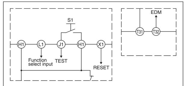
• Wiring for Auto-reset mode and the EDM function enabled
