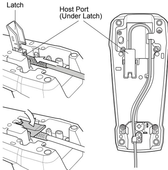
**Important:** Be sure that the interface cable is pushed all the way into the host port before you close the latch.
