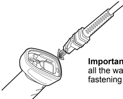
**Important:** Be sure the interface cable is pushed all the way into the connector before closing and fastening the lock plate.
