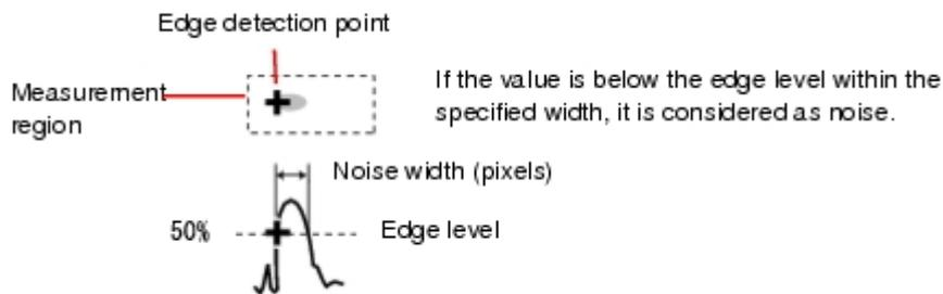
When points are mistakenly detected as edges due to noise, increase the color difference value.
