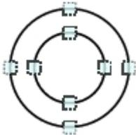
Points are displayed on the top, bottom, left, and right of both the inner and outer circles.
