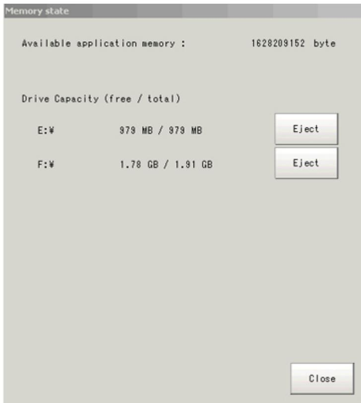
3. To remove the USB memory, tap the [Eject] button.
