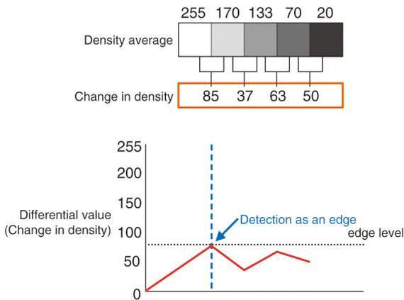
With an image with low contrast, the differential method is suitable as it normalizes the differences between the neighboring pixels for processing.
