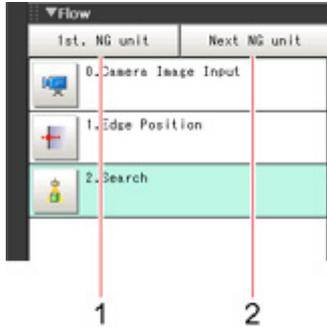
1. Moves to the top processing unit with an NG error.
