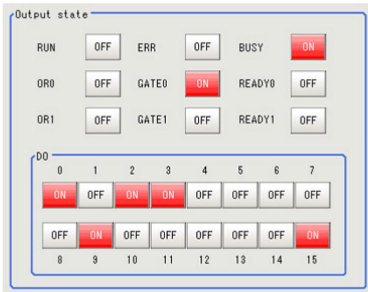
When switching between "ON"/"OFF" is performed, the changed contents are displayed on the monitors of external devices. Please verify it.
