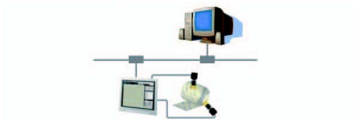
Note that the physical storage location of the data, such as the set data and the data save location, is on the controller side.
