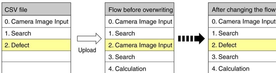
In such a case, the processing item for Unit 3 will be changed from Camera image input to Defects/ Contamination. The parts that do not exist in the CSV file (4. Search processing item and 5. Calculation processing item in the flow) will not change.
