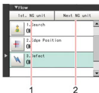
1. Moves to the top processing unit with an NG error.
