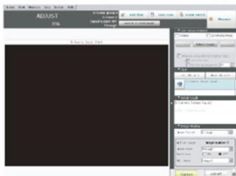
Screen for confirming measurement status and for performing adjustment. When the power is first turned on, the ADJUST window is displayed after the Language Setting window. To set the measurement conditions, move to the Edit Flow window. If there is no problem with the measurement conditions, move to the RUN window.
