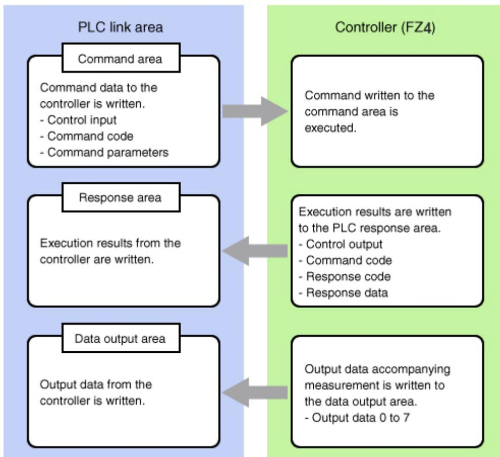
When using PLC Link, it is necessary to specify PLC Link with the communication module.
