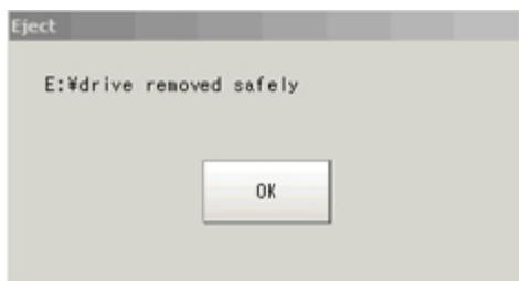
If the removal failed, wait until the USB is no longer accessed and then try removing the USB again.
