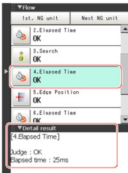
4. Adjust the parameters of the processing units that are taking time.
