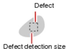
Increasing "Defect size" allows for shortening of processing time, but this will reduce measurement accuracy.
