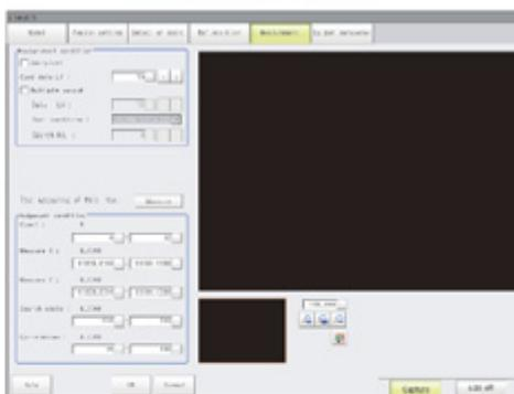
Window for setting conditions for processing units (processing items registered in the scene) set in the flow. This window can also be displayed directly from the Main screen (ADJUST window).
