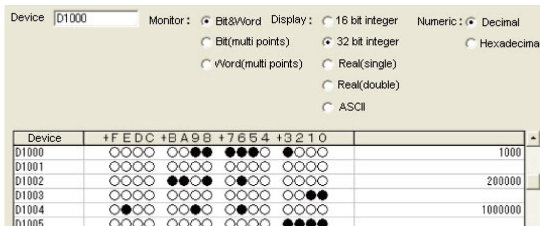
\*: Data is stored to the PLC I/O memory as follows for a decimal number per channel.
