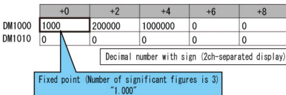
\*: Data is stored to the PLC I/O memory as follows for a decimal number per channel.
