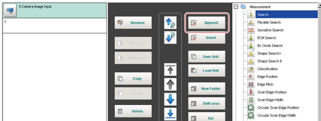
The selected processing item is appended at the bottom of the unit list (flow).
