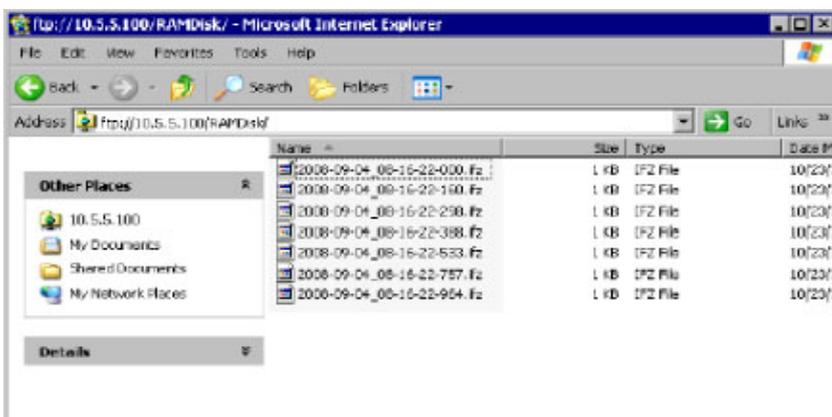
3. In the same way as with normal file operations, logging images can be output from the controller.
