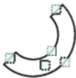
Points are displayed on two lines at both ends of the arcs, on the inner arc, on the outer arc, and inside the closed arc shape.
