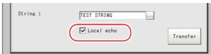
When it is checked, the transfer character string from the device is displayed in the Confirmation window.
