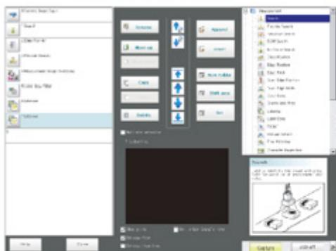
Window for assembling the measurement flow. Flow parts (processing items) are displayed on the right side, and the measurement flow (scene) is displayed on the left side. When the measurement trigger is activated, processing is executed in sequence starting from the top of the flow.
