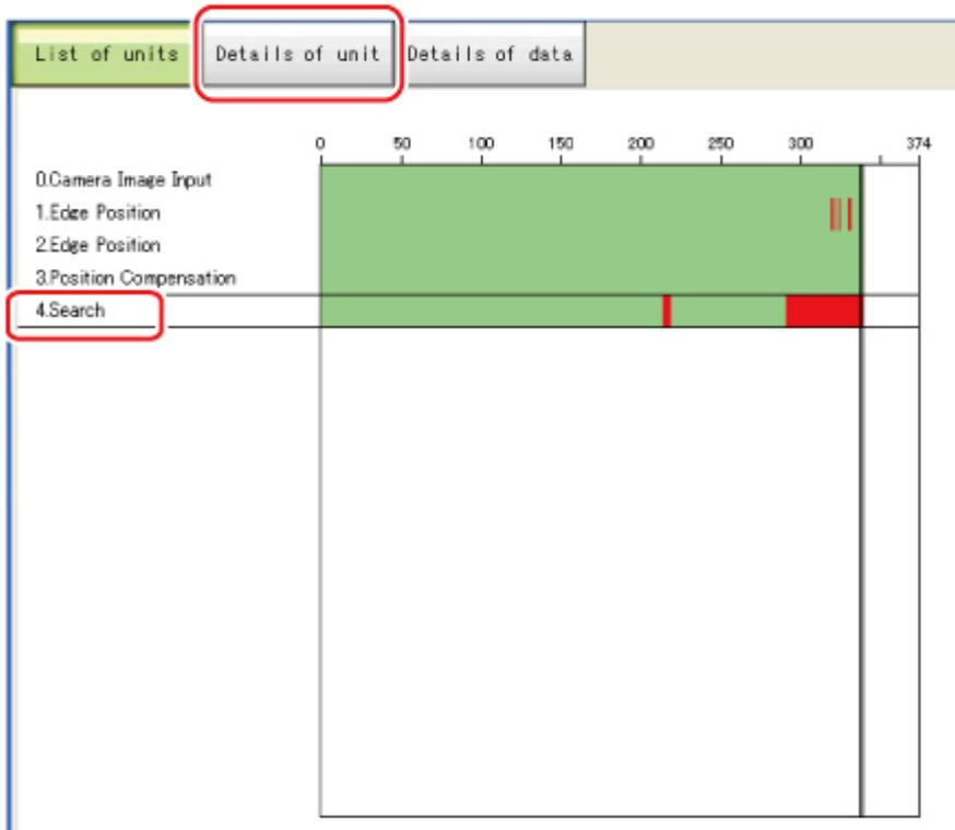
7. The cause of NG is displayed. To check the details of values further, tap [Details of data].
