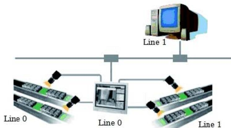
(3) In the non-stop adjustment mode, adjustments can be made remotely without having to stop the line
