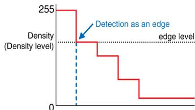
With an image with high noise level or image with blurry edges, the density method is suitable as it allows you to specify the density and color of the edges to be detected.
