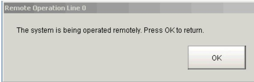
Press the OK button on this window to terminate the remote operation from the controller. The window on which the remote operation is disconnected is displayed on the remote operation PC.
