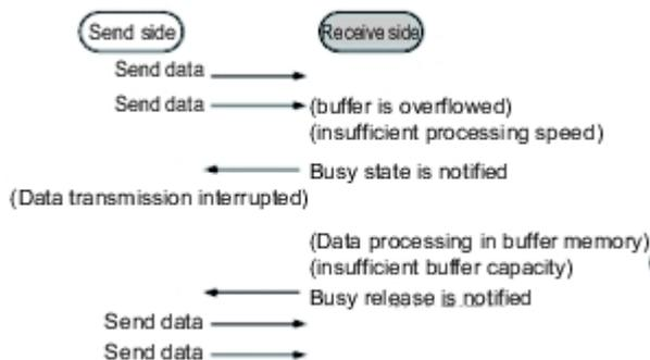
There are two flow control methods: "Hardware Flow Control" and "Software Flow Control". With this product, "Software Flow Control" is used to adjust transmission speed.
