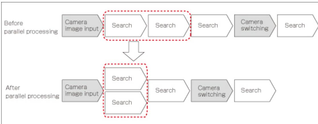
Processing items supporting the aforementioned parallel processing are specified below. You can improve the takt time effectively by combining the applicable units using an ingenious processing flow.
