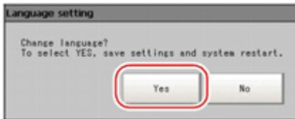
The setting is saved in the controller and the system automatically restarts. After the system restarts, the language switches to the selected one.
