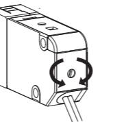
Turn the focus adjustment screw with a force of 60 m N·m or less. Turning the adjustment screw with greater force may damage it.
