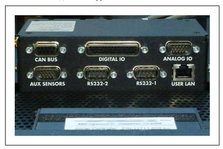
Figure 9-9 Upper Front of Core, Showing RS232 Ports
