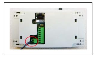
Figure 5-19 VDC Connection on Back of Box Body (Circled)
