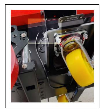
Figure 9-15 LD-250 Front HAPS Cable Routing Behind the Speaker Mount
