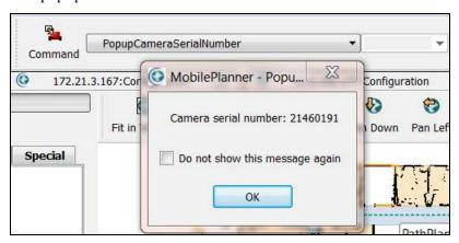
Figure 6-13 Getting the Camera Serial Number
