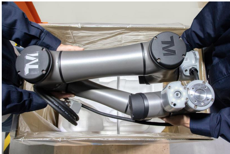
Figure 75: Moving the Robot Arm (2/2)
