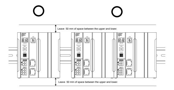
When you install devices other than the UPS on the left or the right of the UPS, leave the space specified by each device.
