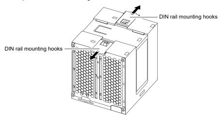
**2.** Hook the "DIN rail mounting groove" in the back of the UPS onto the DIN rail. Put a hook on the groove on one end (①), and put the other hook on the groove on the other end (②).
