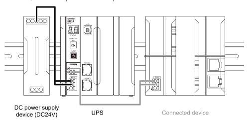
**2.** Connect the input cable to the DC power supply device.
