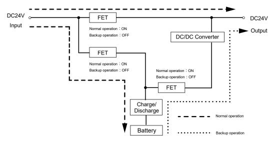
\*In normal operation, 24 VDC is output as-is for charging the battery and from the input power supply. If the 24 VDC from the input power supply becomes lower, the operation automatically switches to backup operation, and 24 VDC is output from the battery.
