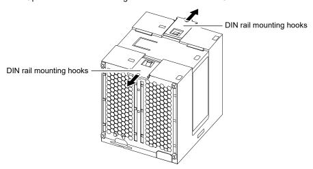
**2.** Use the screw holes of the "DIN rail mounting hooks" to fix the UPS to the floor or wall with screws.
