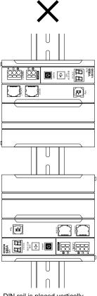
DIN rail is placed vertically
