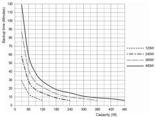
The smaller the capacity of connected devices becomes, the longer the backup time becomes.
