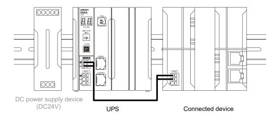
**2.** When using the UPS monitoring software or the I/O signal, connect the unit to the target device with a connection cable. For details about the connection procedure, see "5 Maintenance and inspection", and "6 To perform shutdown processing of the devices when a power failure occurs".
