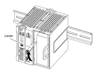
**4.** Insert a tool such as a screwdriver into the hole (the clamp that keeps the battery in place) located on the top of the main body and push the battery out a little toward you.
