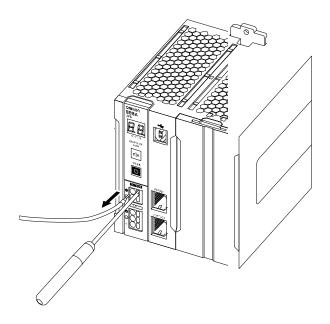
**2.** Pull out the flat blade screwdriver.
