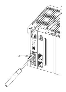
${f 3.}$  Pull out the flat blade screwdriver. Then, the cable is locked.
