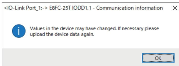
In that case, perform **Load from Device** to check that the expected values are set to parameters if necessary.
