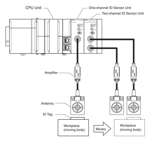
**Note** The above example uses one One-channel ID Sensor Unit (CJ1W-V680C11) and one Two-channels ID Sensor Unit (CJ1W-V680C12).
