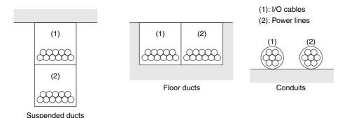
If the same ducts must be used, use the shielded cables to increase resistance to noise. Connect one end of the shield to the ground terminal when you use the shielded cables.
