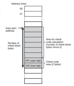
When the Data Check command is executed to verify the data, the CRC code is calculated for the area to calculate and compared with the data in the check code area. If the calculated code is the same as the data in the check code area, the Command Normal End (\*\_Ch1\_NormEndSta, \*\_Ch2\_NormEnd-Sta) in Unit Status will turn ON.
