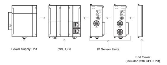
Use the following procedure to connect an ID Sensor Unit.
