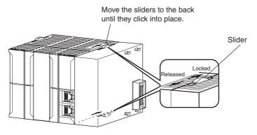
**3** Attach an End Cover to the Unit on the right end of the Rack.
