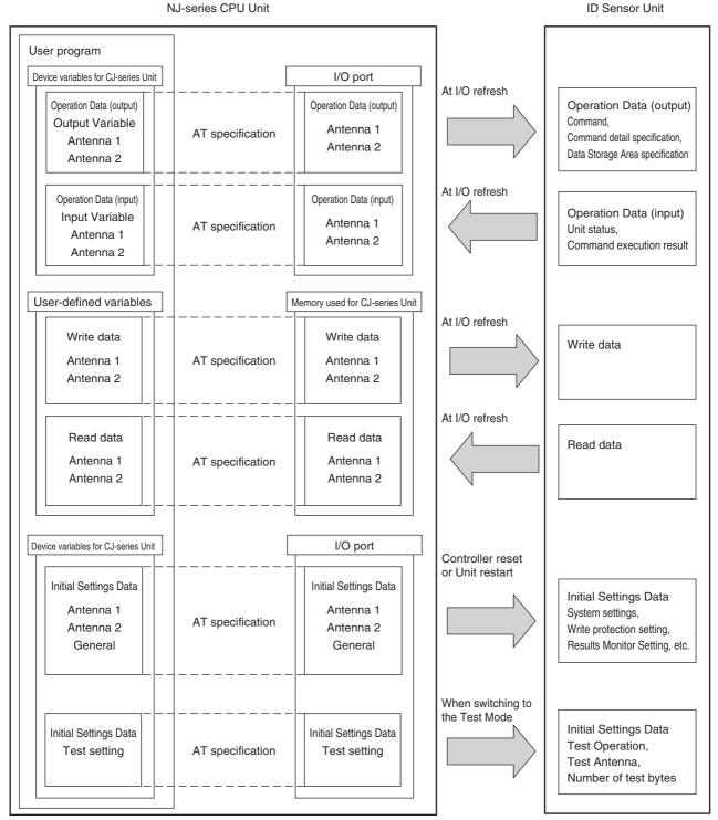
Note The CJ1W-V680C11 has no Antenna 2, so there are no I/O variables and Initial Settings Data for Antenna 2.
