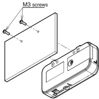
The unit screw hole depth is 4 mm. Be careful not to tighten the screw for more than 4 mm.
