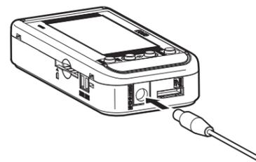
(2) For AC adapter, connect the AC plug into an outlet (100 VAC to 240 VAC). For DC cable, connect the cable with white line to the power supply (24 VDC±10%) and cable without a line into the 0 V.
