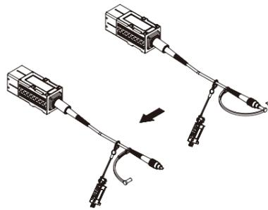
(2) Connect the fiber cable and calibration ROM with the Sensor Controller. Mount the fiber cable in the direction where the protruding portion of the fiber connector and the groove portion of the fiber adapter are aligned. Align the groove portion of the fiber adapter with the protruding portion of the fiber connector, and rotate the screw portion clockwise while pushing it.
