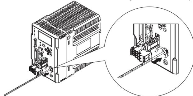
(3) Cleaning of the end face of the fiber connector of the sensor head side
