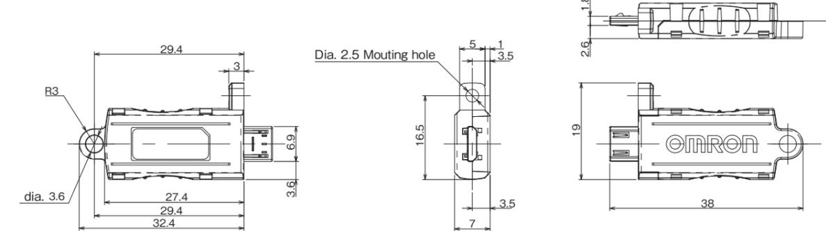
\* Included in the Sensor Head (ZW-S5010/S5020/S5030). Be sure to use the Sensor Head and Calibration ROM of the same serial numbers.
