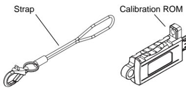
(2) Mount the calibration ROM on the sensor head.
